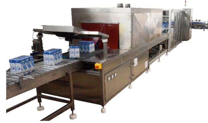
Automatic High Speed Wrap Around Sealer With Shrink Tunnel
